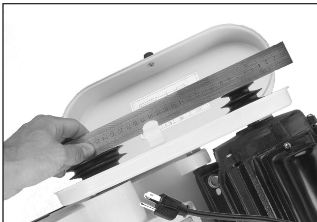
Figure 12. Checking pulley alignment.
